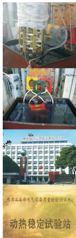
开关做动热稳定试验
